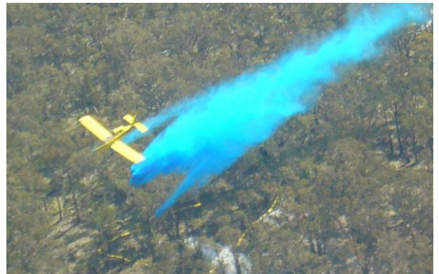
The AT-802F delivers "Thermo-Gel®, 38 seconds viscosity.
