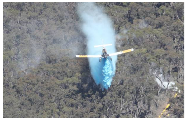
The PZL M18B releases 2200 litres of Thermo-Gel®, at 38 seconds viscosity.
