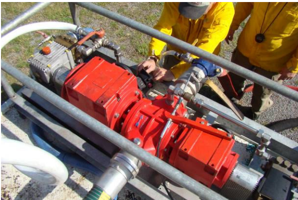
The in-line Fire Dos®. proportioner.
